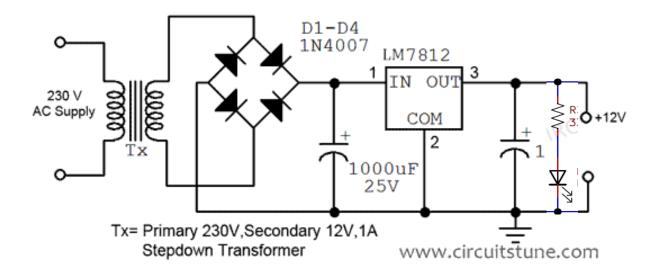
A transformer(Tx=Primary 230 Volt, Secondary 12 Volt , 1Amp step down transformer) is used to covert 230V to 12V from mains. Here used a bridge rectifier made by four 1N4007 or 1N4003 diode to convert AC to DC . The filtering capacitor 1000uF,25V is used to reduce the ripple and get a smooth DC voltage. This circuit is very easy to build. For good performance input voltage should be greater than 12Volt in pin-1 of IC LM7812. Use a heat sink to IC LM7812 for safeguarding it from overheating.
